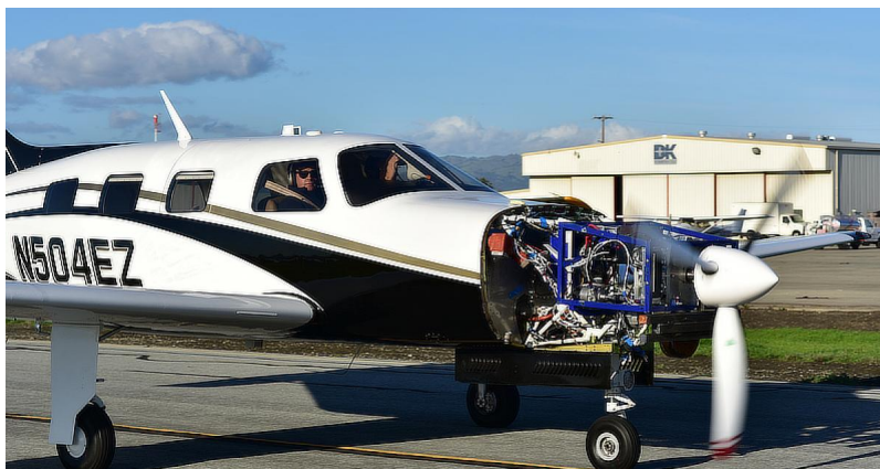
Figure 3.6: ZeroAvia's Piper Matrix with replaced powertrain shown (nose is closed during flight)
